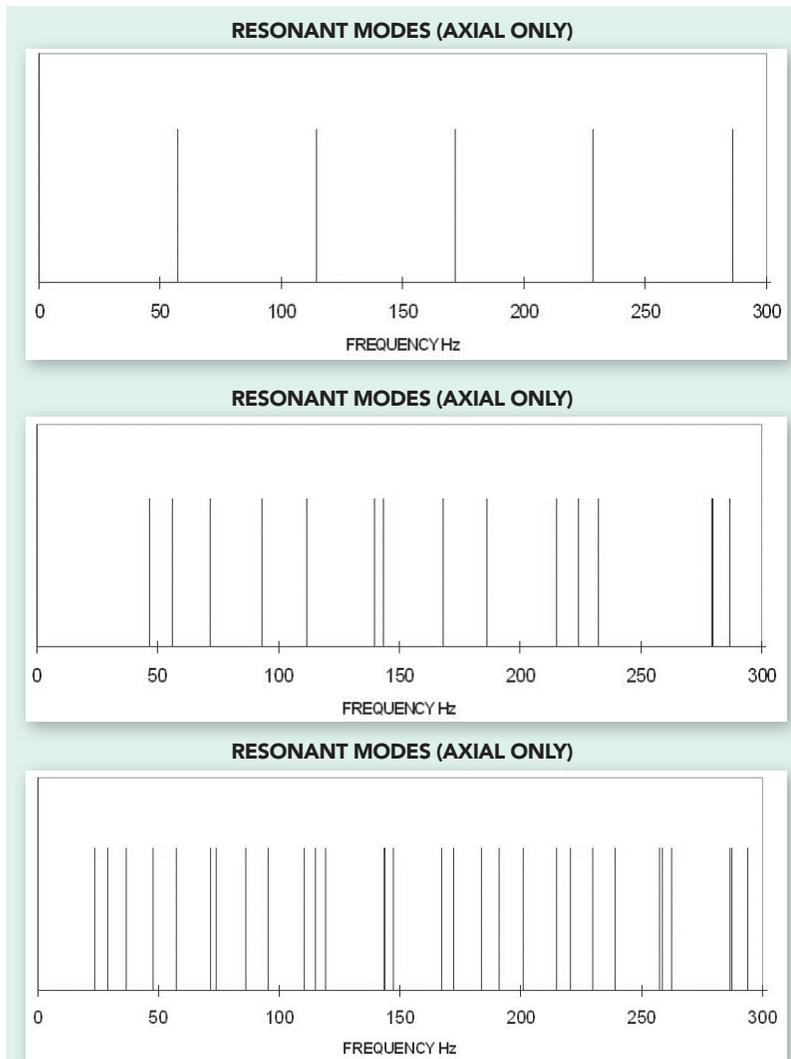
**Fig. 1. Modal density can be increased by selecting the right proportions for the room dimensions. Top: 27m3 room with 1:1:1 ratio. Middle: 27m3 room with 1.54:1.28:1 ratio. Bottom: 200m3 room with 1.54:1.28:1 ratio.**
