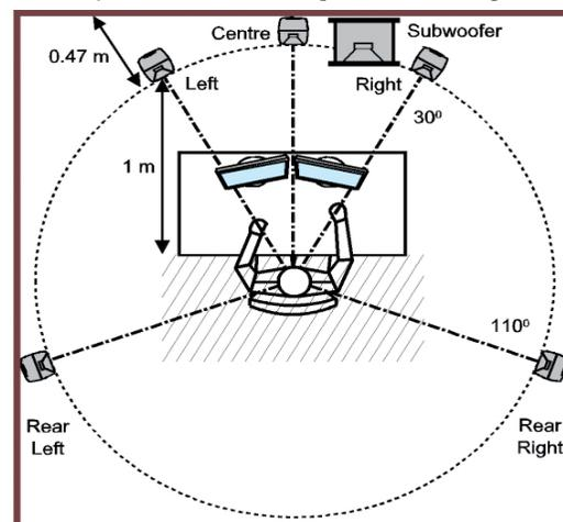
**Fig. 4. 5.1 monitoring system in a 3m x 4m rectangular room without any acoustic treatment.**
