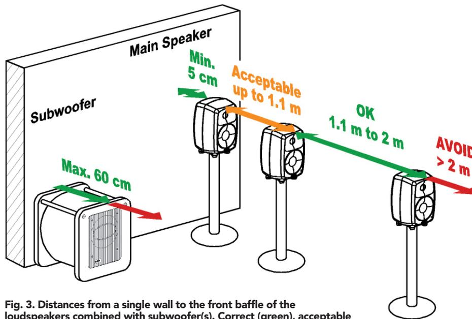
**Fig. 3. Distances from a single wall to the front baffle of the loudspeakers combined with subwoofer(s). Correct (green), acceptable (orange) and avoid (red).**
