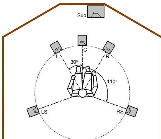
Figure 4: ITU R BS.775-1 speaker placement with each main speaker placed at least 1.1m from the wall behind.
