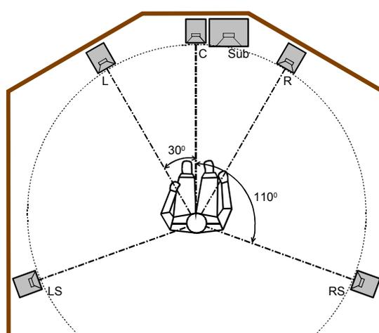
Figure 3: ITU R BS.775-1 speaker placement with each main speaker placed against a wall. (hemispherical loading)
