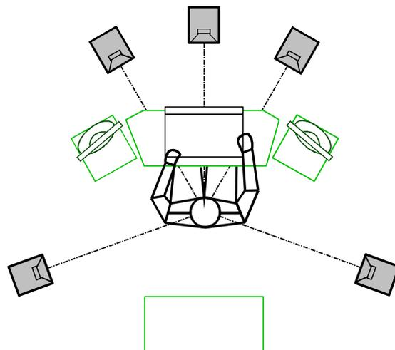
Figure 2: Example of a symmetrical equipment layout for a multichannel control room.
