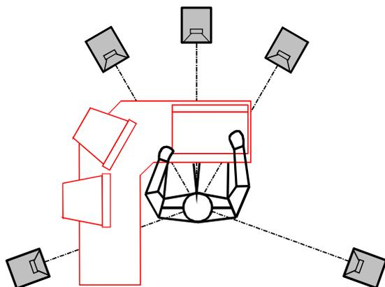
Figure 1: Non-symmetrical equipment layout leading to compromised sound field.
