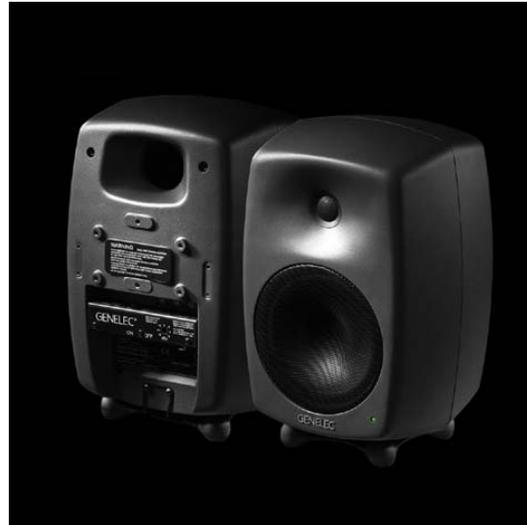
enclosure starts to become directive when the baffle dimensions are comparable to  $1/3 - 1/2$  of the wavelength. To minimize this effect as well as diffraction at higher frequencies, the enclosure was designed with rounded edges and curved surfaces all around. This translates in an even more natural sound reproduction in the critical midrange region.
