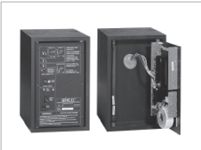
Two channel amplifier is housed in the speaker cabinet
