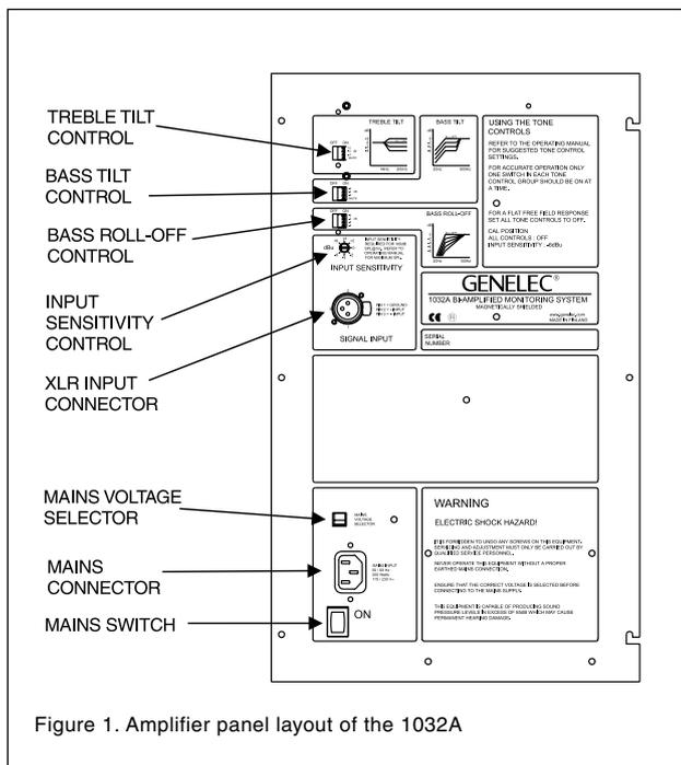
Figure 1. Amplifier panel layout of the 1032A
