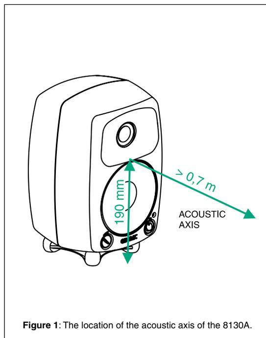
Figure 1: The location of the acoustic axis of the 8130A.
