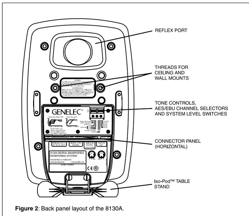
Figure 2: Back panel layout of the 8130A.
